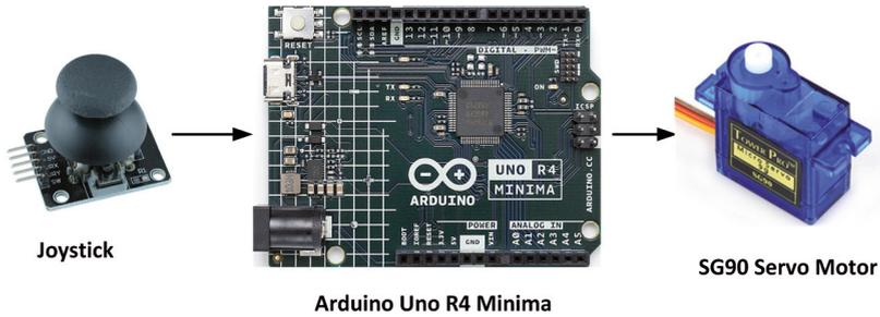
Figure 12.6: Block diagram of the project.
