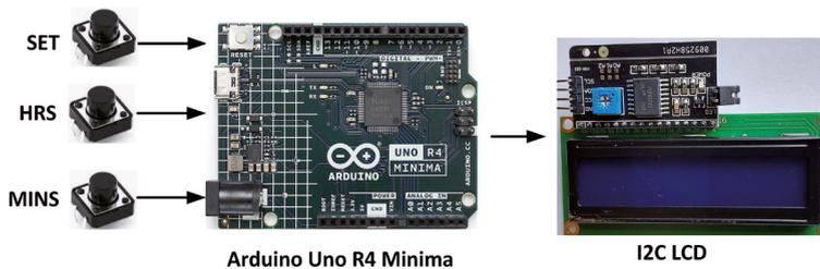
Figure 5.18: Block diagram of the project.
