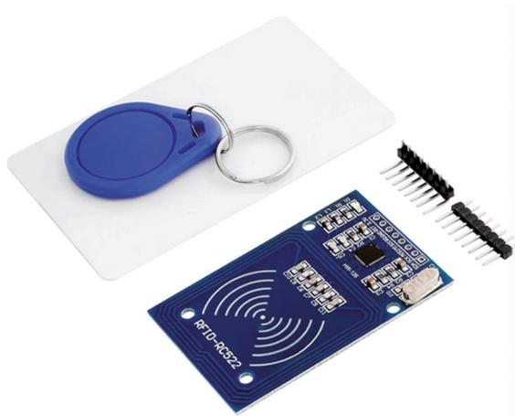
Figure 7.1: RFID reader and tag.
