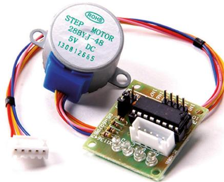
Figure 12.9: 28BYJ-48 stepper motor and driver board.
