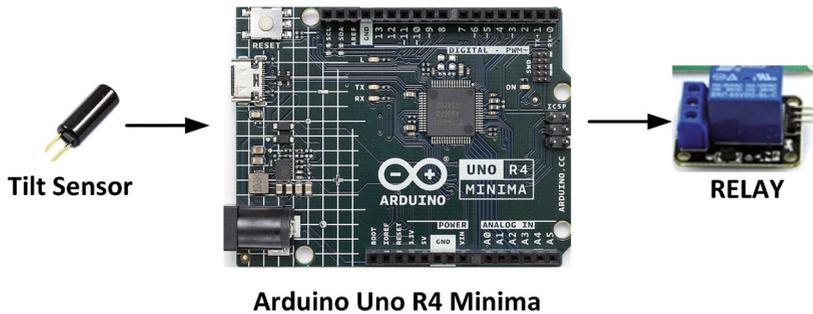
Figure 6.16: Block diagram of the project.
