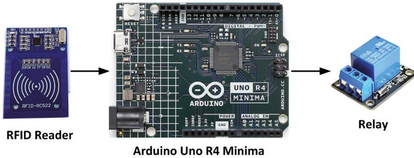
Figure 7.5: Block diagram of the project.
