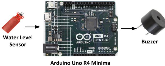
Figure 6.26: Block diagram of the project.
