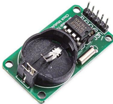
Figure 9.1: The supplied RTC module.
