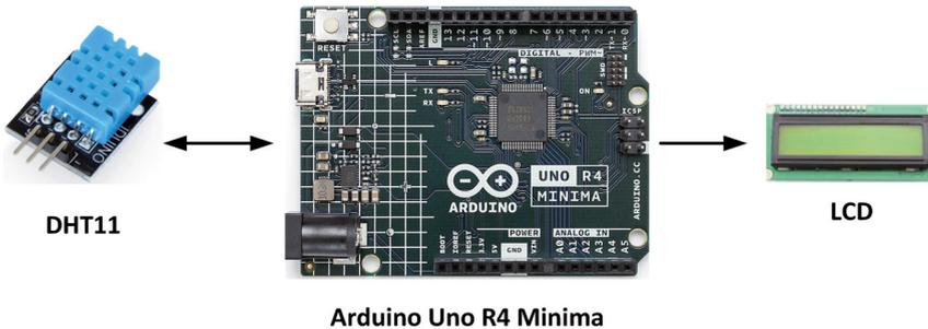
Figure 6.37: Block diagram of the project.
